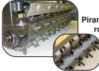
Piranha offers 3 rotors to choose from: 2" Sabre tooth rotor, aggressor tooth carbide rotor (which is 50% more aggressive, takes 25% less power than our discontinued carbide button tooth), and the construction rotor which is excellent for laying down gravel or processing soil.
