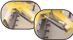
**Manual or Hydraulic Angle:** You may choose either manual or hydraulic angle. Tractors are operated off the rear SCV. Skid steers feature an electric solenoid, which directs hydraulic oil off the main hydraulic drive to turn the angle cylinder. Hydraulic angle not available on PXT & PXS models.
