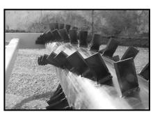
MaxiMizer Tooth: This 3 1/2-inch tooth is a case-harden, beveled turned tooth design needing minimal power to get the job done. You may operate the tooth in directional or bi-directional silage processing (forward or reverse) This spiral design lets only one tooth hit the pile at a time instead of multiple teeth hitting at the same time, robbing you of power and performance.
