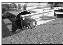
Hydraulic Direct Drive: Cut costs along with cutting down on weight. This simple direct drive system is an easy low-cost way of transferring power to the rotor. Direct drive also reduces weight.
