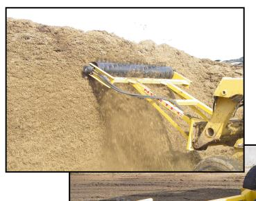
Model: **NORTEC FA605D** Width of cut: 6' (182.88cm) **Boom Reach:** 7' (213.36cm)
