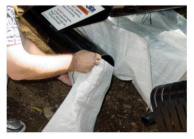
Rotating the **BAGRR<sup>TM</sup>** upwards causes the material in the loading tubes to fill the bags.
