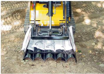
The bags fall off the  $BAGRR^{TM}$  ready to be tied closed and put to use. Average loading time is approximately 30 seconds\*.
