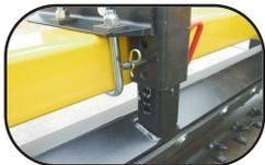
The new, stronger material bar is equipped with a positive locking system. This system adjusts quickly, easily and accurately - no tools required! Heavy-duty fabricated design for trouble-free operation. Material bar belting is made of high-quality multi-ply belting.
