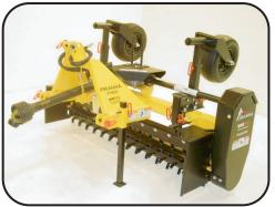
Industry Exclusive \*Flip-Up Gauge wheels \*Extender In/out gauge wheels \*Quick-Change Rotors \*Aggressor Tooth \*Adjustable Side Shields
